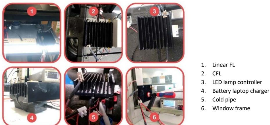
Figure 21. TEG system attachment to the various thermal source objects
