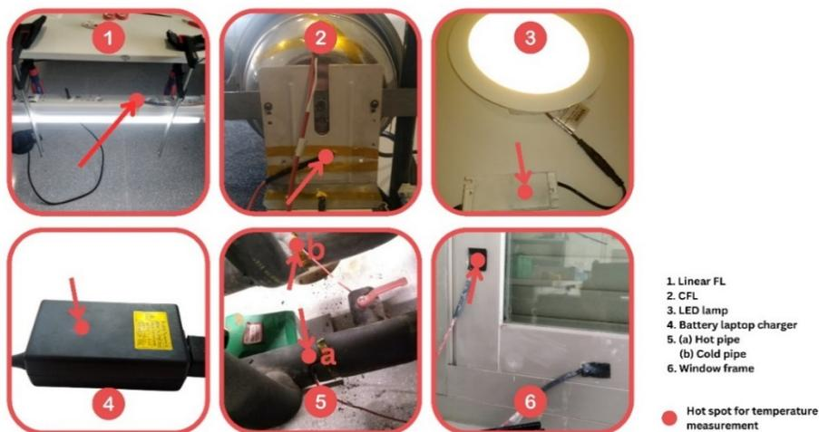
Figure 5. Hot spot where temperature recorded for each object
